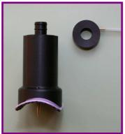
The mechanical actuator has a rolling diaphragm to ensure low friction and a "donut" O ring connection to the pressure line. This is designed to pull away without damage to the system if the subject becomes excitable. The standard pin diameter for large animals is 1mm. Other sizes, and a three pin configuration are also available on request. The actuator is supplied with mounting straps and boots and a dummy set for the contra-lateral limb.
